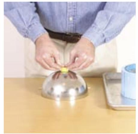
**30. Attach a pouring gate to the dome.**
