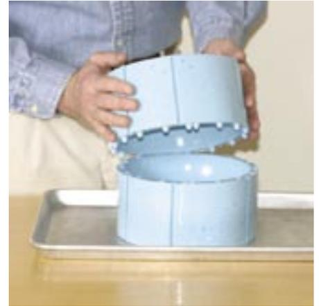
**42. Put the mold halves together.**
